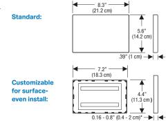
\*NOTE: Customizable surface-even cover plate accepts typical wallcovering materials to disguise the service opening. Minimum finished wall is ≥3/4" (1.8 cm) plus cover thickness up to a maximum of 2" (5 cm) total.
