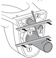
**4** Add dimension X and 1/8". Using that dimension, mark a line on the pipe measuring from the hub side. Cut off the pipe at the line with a pipe cutter.
