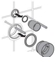
2 Insert discharge pipe into the pipe hub in the wall. Place a straight edge flush against the wall and mark a line on the pipe. Fit finned rubber seal onto flush pipe. Repeat same procedure for discharge pipe.
