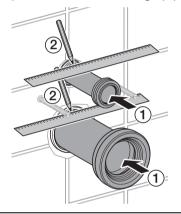
**3** Place discharge pipe with gasket into waste outlet of bowl. Also place flush pipe with fin gasket into inlet of bowl. Then mark a second line on both pipes.
