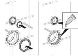
8 Remove protective sleeves from mounting rods. Determine protruding rod length for bowl installation. Install both pipes into the hubs in the wall.
