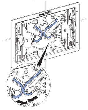
**3** Remove the tension wedges.
