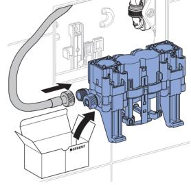
Check that the pipe bracket clip is aligned parallel to the flush valve.
