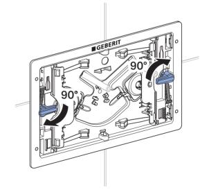
20 Secure the distance bolts with tension wedges.
