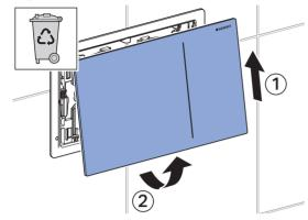
2 Mount the new Geberit actuator plate Sigma70.
