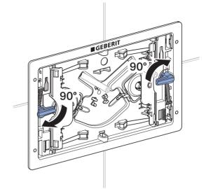
Secure the distance bolts with tension wedges.
