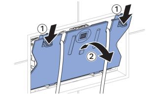
**7** Remove the defective pneumatic hose.
