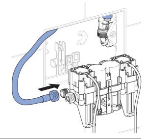
**13** Check that the pipe bracket clip is aligned parallel to the flush valve.
