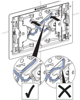
**24** Mount the Geberit actuator plate Sigma70.
