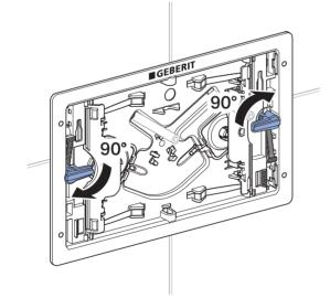
Secure the distance bolts with tension wedges.
