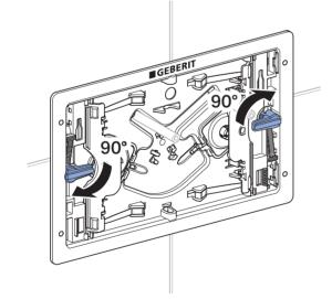
Secure the distance bolts with tension wedges.
