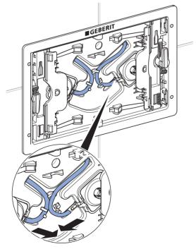
3 Remove the tension wedges.
