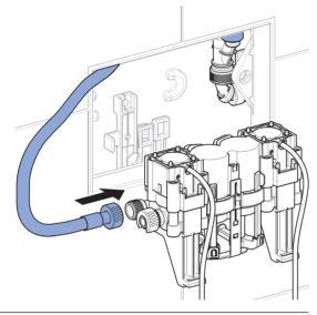
20 Check that the pipe bracket clip is aligned parallel to the flush valve.
