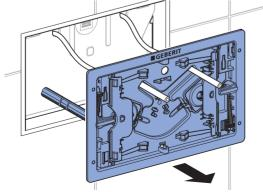
6 Release the protection plate and detach.
