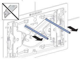
Connect the pneumatic hoses in the mounting frame.
