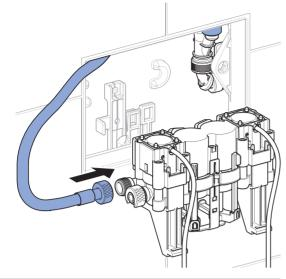
Check that the pipe bracket clip is aligned parallel to the flush valve.
