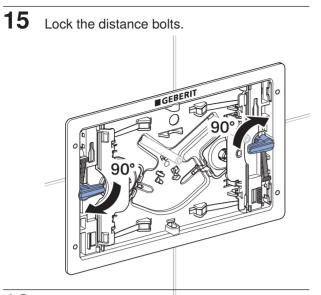
Secure the distance bolts with tension wedges.
