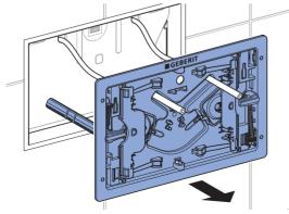
6 Release the protection plate and detach.
