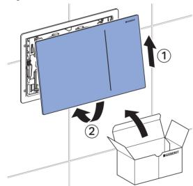
Cleaning the filter (Geberit Sigma concealed cistern 8 cm to year of manufacture 2015)
