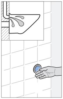
To activate: Place hand 3/4" to 4" (19mm to 102 mm) in front of sensor for approx. 0.5-1 second for a full flush and for 2 seconds or longer for a partial flush.
