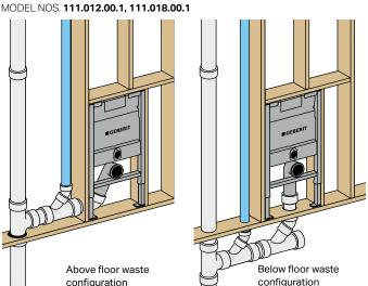
IMPORTANT: CARRIER FRAME MUST BE MOUNTED FLUSH WITH WALL FRAMING FOR PROPER INSTALLATION.
