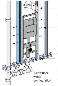
Recommended lateral reinforcement of plywood or drywall for thinner gauge steel, at least 12" (30cm) height.
