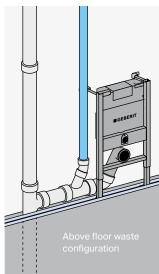
Note: All carriers can be installed as pre-wall (in front of solid wall) and can also accommodate both above and below floor waste lines.
